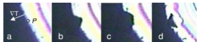
FIG. 3. Sequence of polarized photomicrographs of the head and its trailing thin nematic layer invading the AFM-scribed square on cooling. (The tail remains outside the image). (a) Head becoming pinned at point P , corresponding to temperature T_1 ; the temperature gradient is shown. (b) Head continues to move around square. (c) Head begins to advance beyond point P into square at temperature T_2 . (d) Head advances further into square. The 100 \mu\text{m} \times 100 \mu\text{m} AFM-scribed square is outlined, indicating the length scale in the images.
